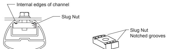
Notched grooves in Slug Nut must run parallel with internal edges of channel
