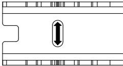
The slotted hole in each of the Lower Brackets will provide enough adjustment to fit a Hilift jack regardless of Cross Bar spacing. Take note of which direction the mount needs to go. Remove the jack, and loosen the 'T' bolt nut, reposition, re-tighten, and try again.
